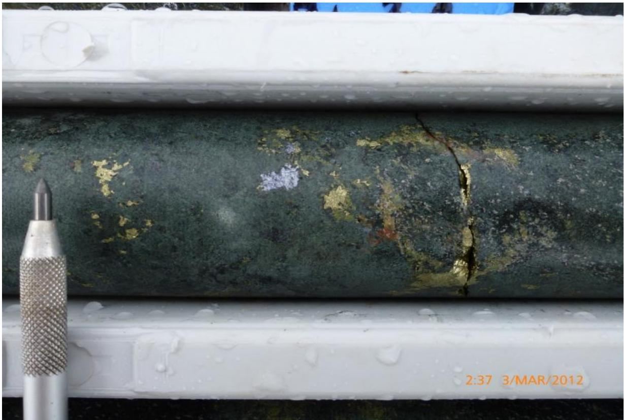
*Figure 2. Zone of intense amphibole rich alteration with associated chalcopyrite and possibly chalcocite in drill hole WTDD002 at 247.5m.*
