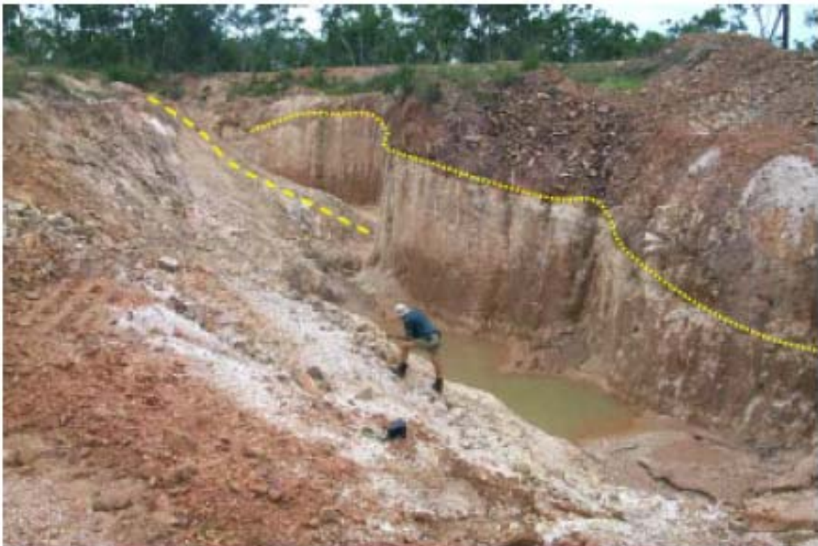
Figure 2: Booths South Pegmatite (North-western Pit). Dotted line indicates hanging-wall contact (source NTGS Report 16).
