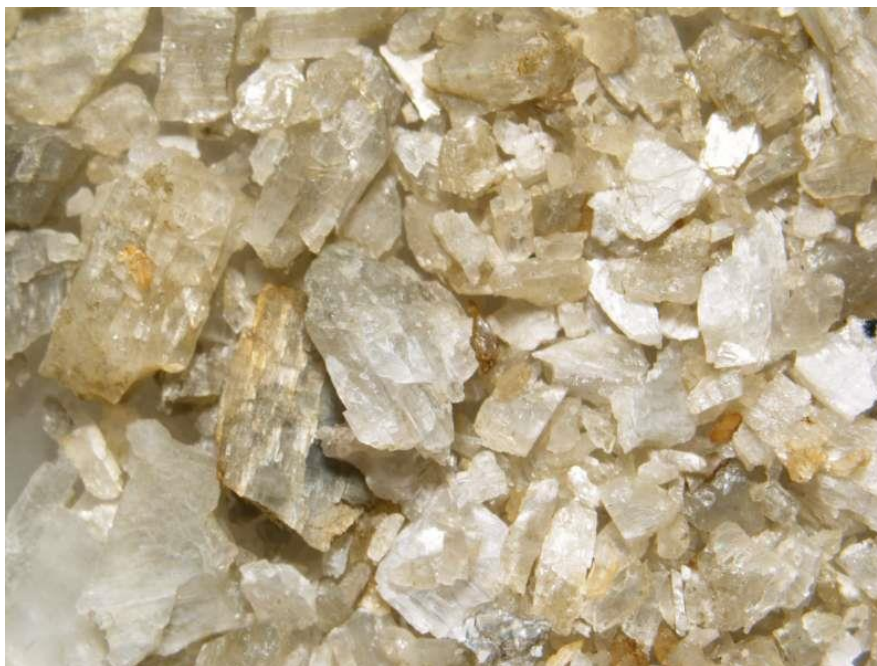
Figure 1. 8.10% Li 2 O Spodumene from HLS Testwork (SG 3.1 Sink).
